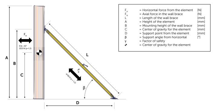
NOTE! The force  $F_N$  can be tensile or compressive.
