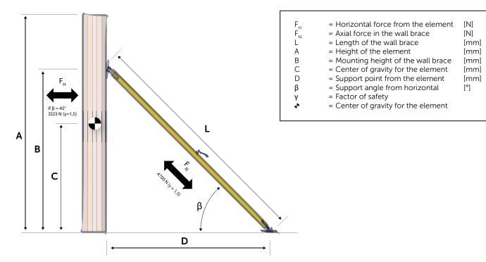
NOTE! The force  $F_N$  can be tensile or compressive.
