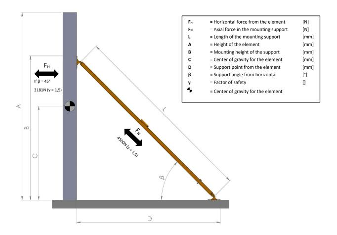
NOTE! The force  $\boldsymbol{F}_{\boldsymbol{N}}$  can be tensile or compressive.
